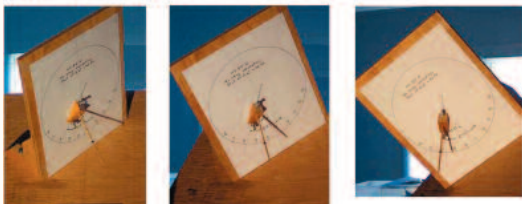
My simple heliodon with F-L dial face. Clockwise, from upper left: overall view, time is peedawn; about 0730; minimum shadow when it lies along substyle; about 0845; about 1130; about 1245, almost the limit for this wall. For all of these photos, the device was set for a solar declination of -33.44°
